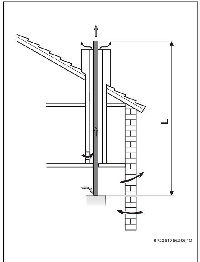
Fig. 15 Configuration B<sub>23p</sub> verticale
